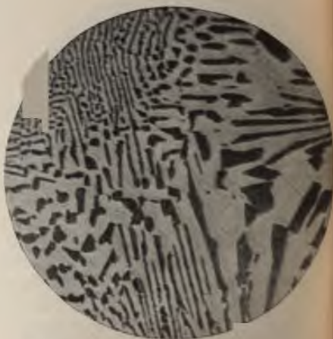
FIG. 17.—ALLOY OF SILVER AND COPPER— EUTECTIC—CU, 28% ; SILVER, 72%. Magnified 600 diameters.
